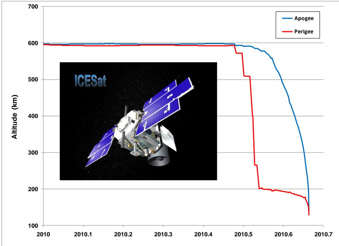
Figure 8. ICESat reentered the atmosphere only 6 weeks after its orbit-lowering maneuvers.
