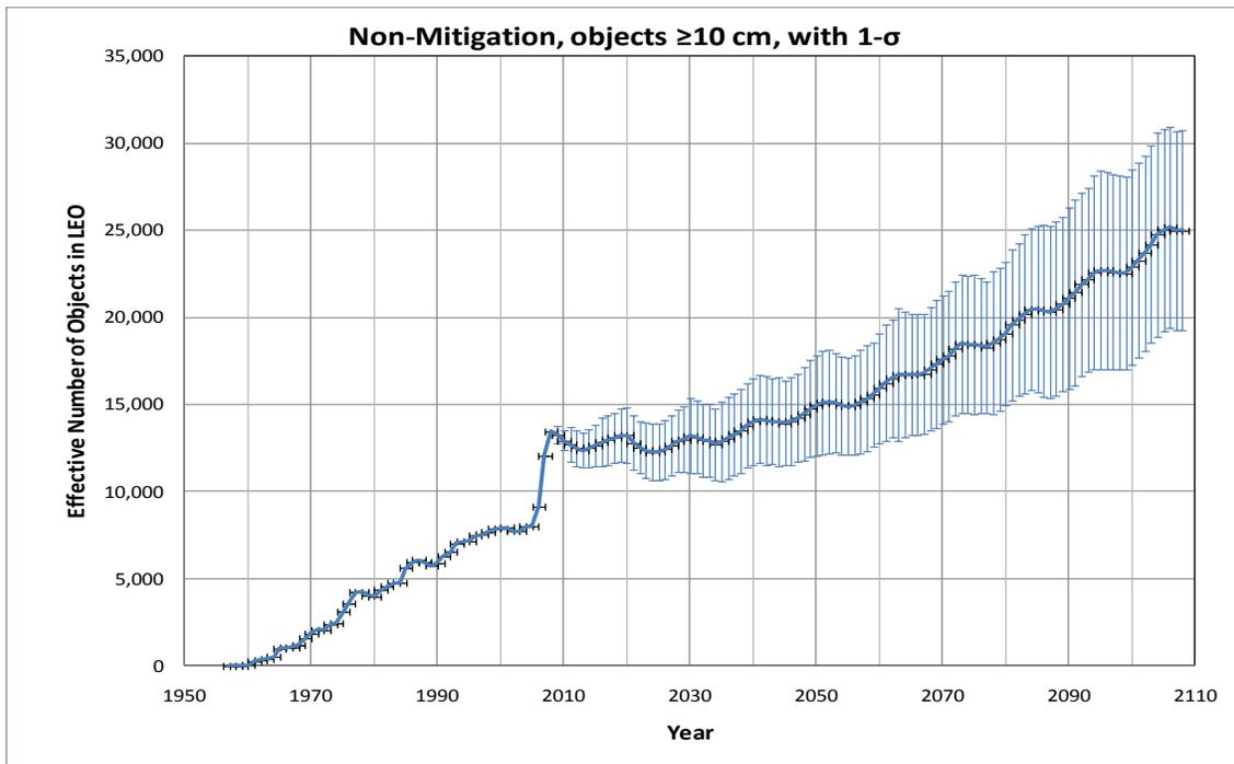
Figure 10. Projected growth of satellite population in low Earth orbit with annual space launches at recent rates and without active debris removal (Source: NASA).
