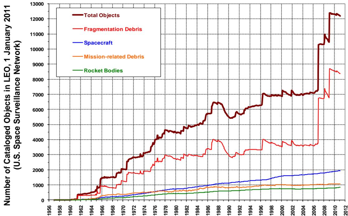
Figure 5. Growth of the cataloged population of objects in low Earth orbit only.
