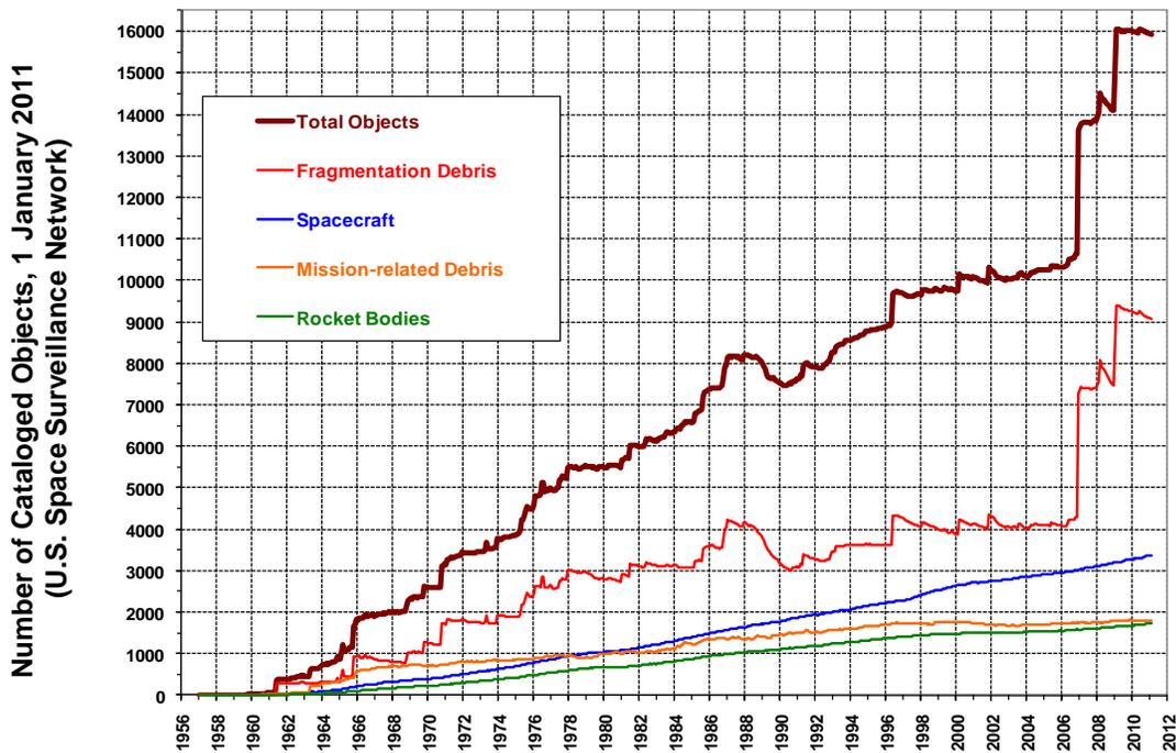
Figure 4. Growth of the cataloged population of objects in Earth orbit. The growth of the cataloged Earth satellite population in just the LEO region is illustrated in Figure 5. This is the most highly congested region in near-Earth space. For objects too small to catalog, the population levels are much higher. For instance, the number of debris between 1 and 10 cm is assessed to be several hundred thousand, and the number between 1 mm and 1 cm is assessed to be in excess of 100 million.
