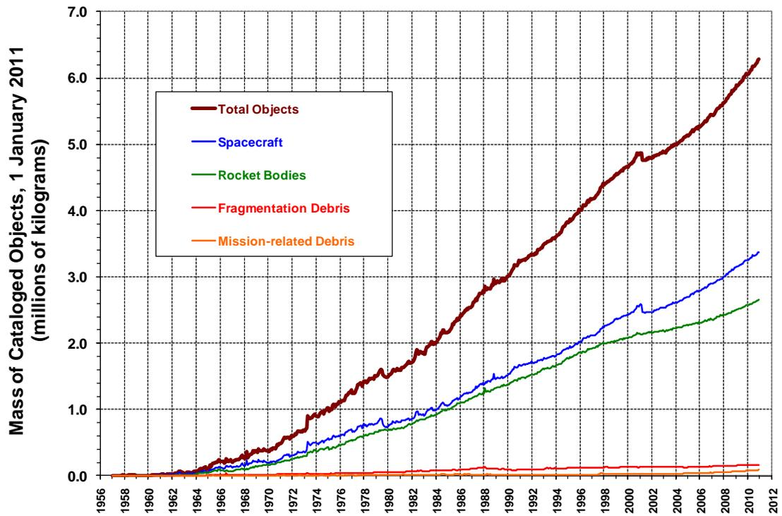
Figure 6. Growth of mass of man-made objects in Earth orbit.
