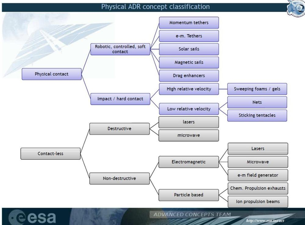
Figure 11. Hierarchy of the principal concepts for active debris removal.
