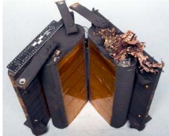
Fig. 4.2-2 After test imagery of HITF12143 a) shield with 9.5cm diameter through-hole, and b) cell close-up with impacted cell on right showing molten material from cell interior that was ejected and deposited on exterior of cell.
