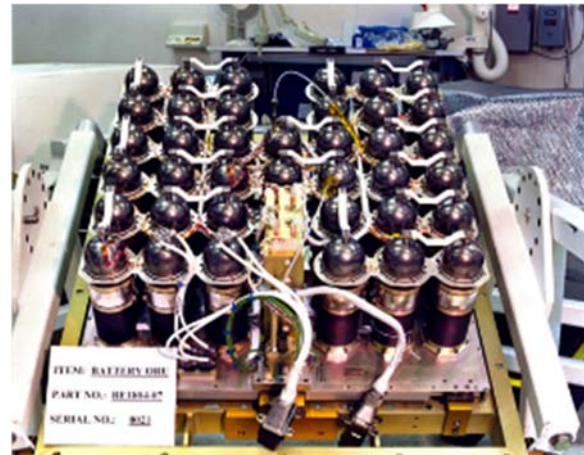
Fig. 4.2-3 a) ISS Ni-H 2 battery ORU and b) ORU subassembly without enclosure.
