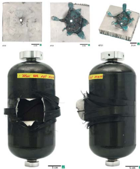
Fig. 8.3-3 Damage on pressure vessel of experiment 4750 (front and side views)
