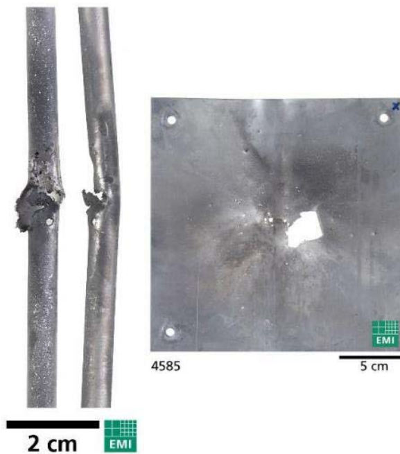
Fig. 10.1-4 Fuel pipe (front and side view) and witness plate damage of Exp. 4585
