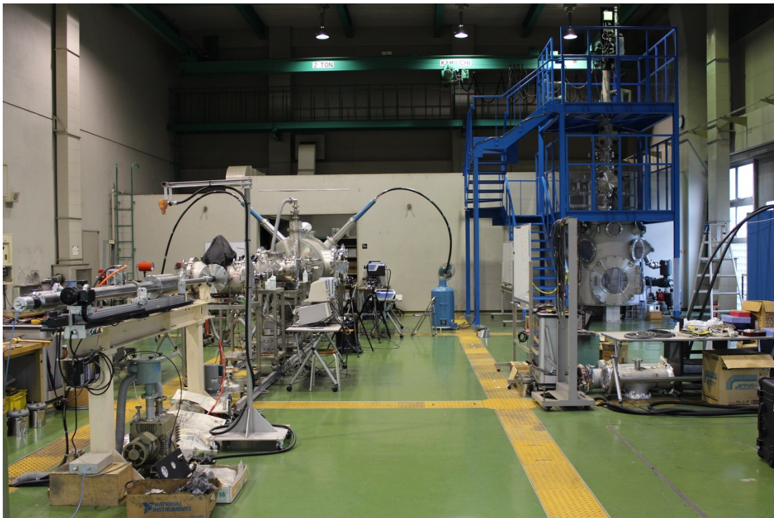
Figure 4.4-1: JAXA two-stage light gas guns: (left) the horizontal accelerator, (right) the vertical accelerator
