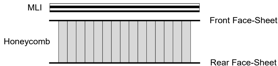
Figure 3.1-9: Standard Single-Honeycomb Panel Structure with MLI
