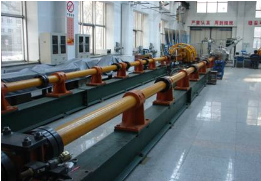
Figure 4.4-8: Two-stage light-gas gun at HIT
