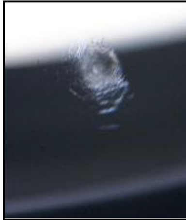
Figure 1.3-1: Meteoroid/Debris impact damage on Service Module Window #7
