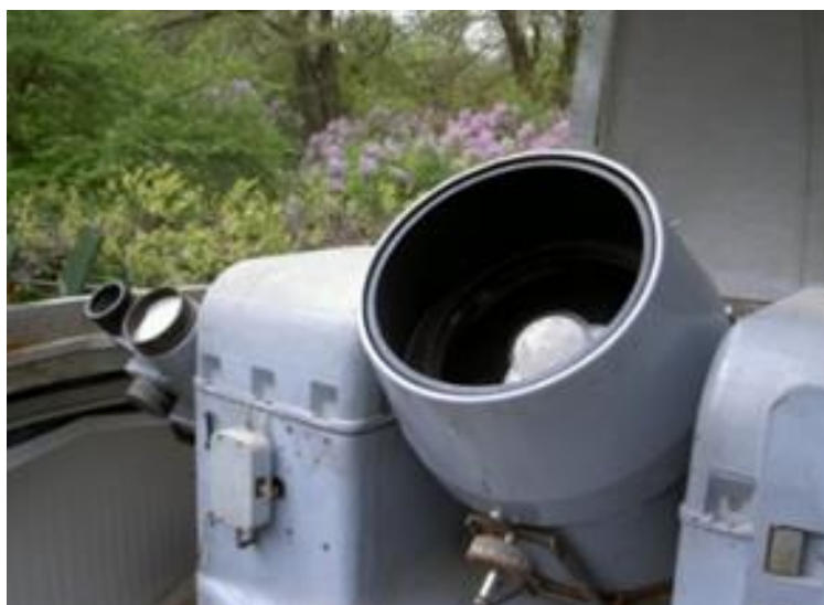
Figure 14: KT-50 telescope of AO ONU. A Maksutov telescope with diameter of 500 mm and focal length of 2000 mm with an alt-azimuth mount. Mounted at the focal plane is a TV-CCD camera Watec-902H2 able to take 50 TV half-frames every second.
