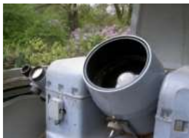
Fig. 6 KT-50 telescope of AO ONU. A Maksutov telescope with diameter of 500 mm and focal length of 2000 mm with an alt-azimuth mount. Mounted at the focal plane is a TV-CCD camera Watec-902H2 able to take 50 TV halfframes every second.
