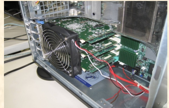
FPGA system for the method has been developed to reduce analysis time to 1/1000.
